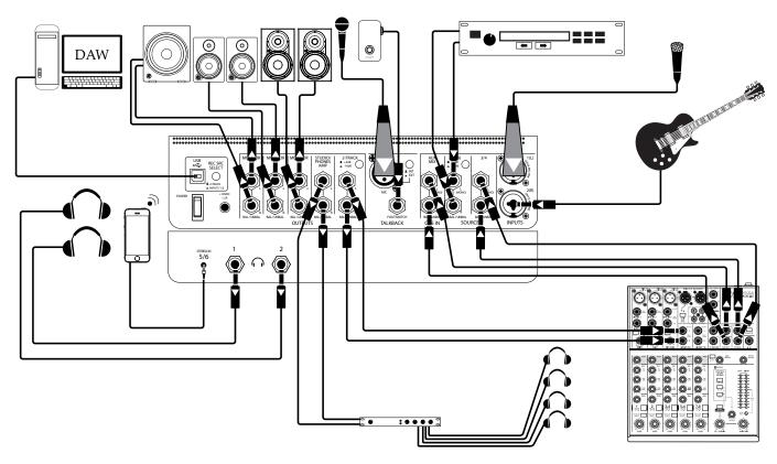
The Big Knob Studio<sup>+</sup> is similar to the Big Knob Studio, but with a few more bells and whistles. No time to waste, let's get started! In this example, a microphone is connected to XLR input 1 (L) and a guitar to 1/4" input 2 (R). The Source Input 3/4 jacks are connected to an external mixer's Control Room (CR) output jacks, playing whatever sounds / sources are fed into the mixer. Likewise, the Cue In (Aux Mix) jacks are connected to the same mixer's Alt 3/4 output jacks.
