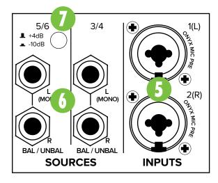
These 1/4" connectors are wired the same as the combo input connectors as seen on the previous page.
